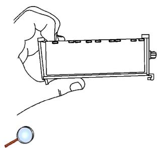
11. On bottom side of plastic bracket assembly, directly below the 2 large, plastic snap features, locate the under cut edge. Pull this under cut edge outward, up and over the side of the module.
