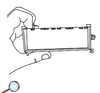
3. Spread the large tang side of the plastic bracket over the edge of the module. The bottom, undercut edge of the plastic bracket will snap over the bottom of the module when fully seated.
